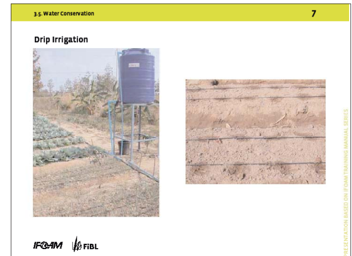
TRANSPARENCY 3.5.3(7): LEFT: DRIP IRRIGATION SYSTEM IN VEGETABLE CULTIVATION, RIGHT: DETAIL OF THE DRIP TUBES (THAILAND)
